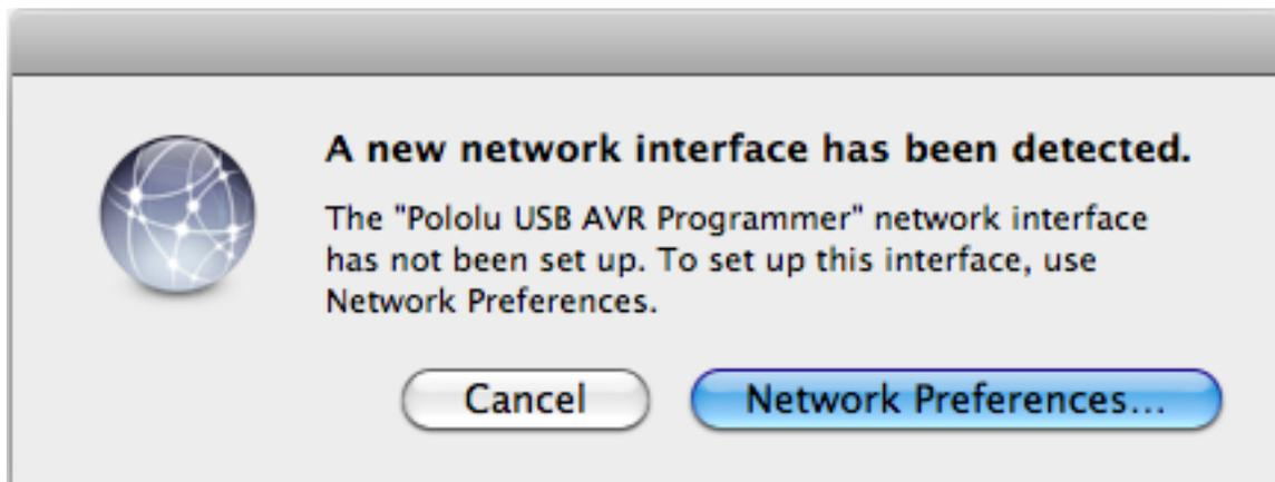
In a Terminal window, type `ls /dev/tty.usb*` and press enter. You should see 1–3 new entries of the form `tty.usbmodem<number>` (e.g. `/dev/tty.usbmodem00022331`). These entries represent virtual serial ports created by the programmer or Orangutan SVP.
